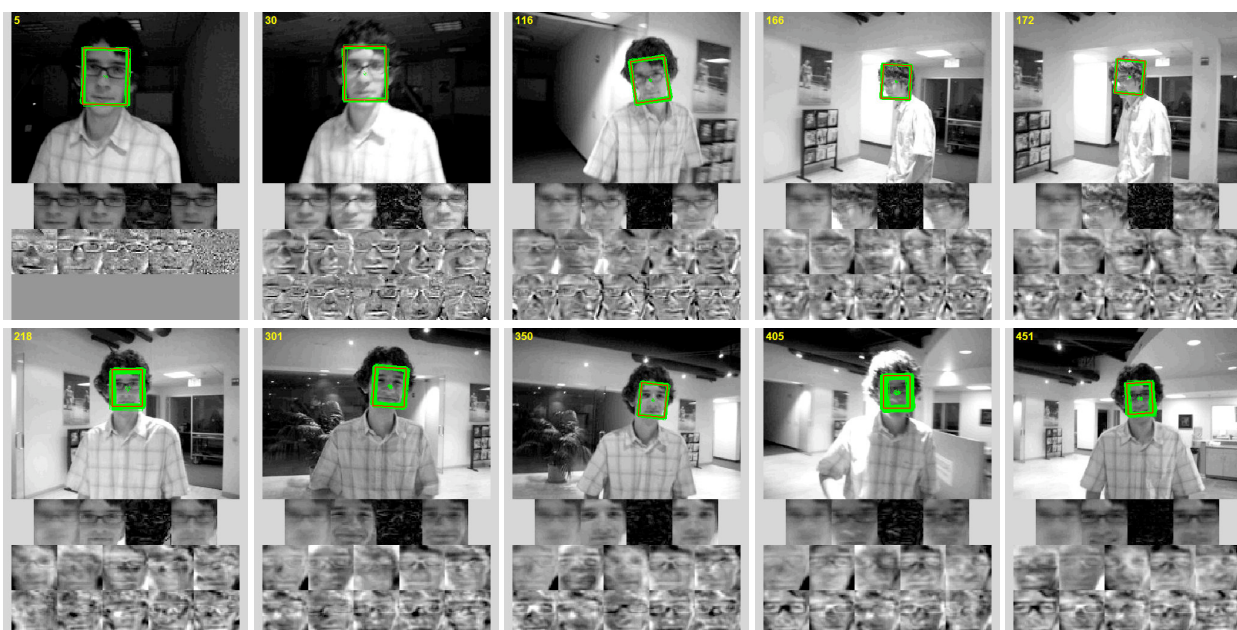
Figure 6: A person moves from a dark to a bright area, undergoing large lighting and pose changes. The images in the second row show the current sample mean, tracked region, reconstructed image, and the reconstruction error respectively. The third and fourth rows show the top 10 principal eigenvectors.
