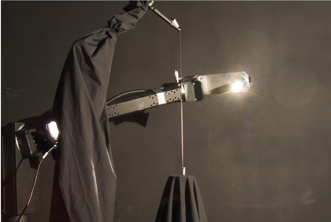
Figure 3.1: An image showing the thread BRDF measurement setup using the UCSD Hemispherical Gantry. It shows a vertically suspended thread sample being illuminated by a light source.
