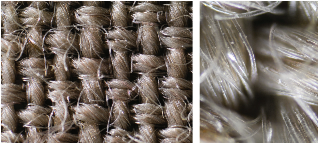
Figure 2.5: Microscope images of the wool flannel fabric. The fabric (left) is made out of one type of thread (spun). The right image shows a closeup of the thread structure where individual wool fibers are visible and their translucency is apparent.
