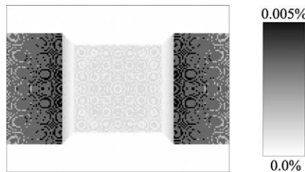
Fig. 15. Difference between the image of area lights approach and point lights approach. The error values are calculated by subtracting the phase image A_0 produced by the simplified point lights approach from the phase image A_0 generated by the area lights approach. It should be noted that the black regions differ less than 0.005% from the area lights approach and the white regions contain even smaller differences. This means that the resulting values are almost zero and thus the two approaches produce nearly the same simulation results.
